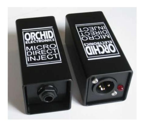
Housed in a strong steel tube 90 X 40 X 40 it has only a jack socket input for connection to the instrument and an XLR output to feed the microphone input of a mixing desk - which can be located many hundreds of metres away if necessary. It must receive Phantom Power from the mixer as it is an active design - a red LED will indicate power present.
